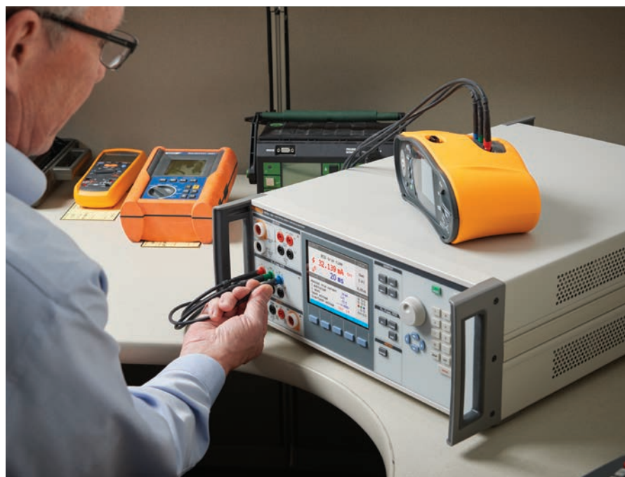
Each 5322A comes with an external R-Multiplier to source resistances of 10 TΩ for testing insulation testers.
